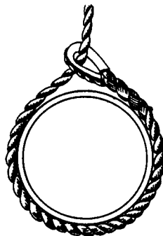
Correct – Use thimbles in the eyes.
